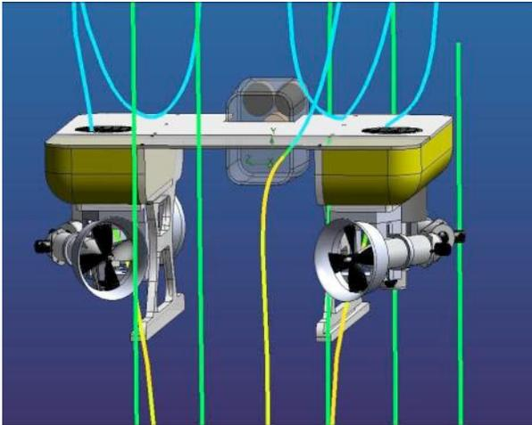
Figure A3. Flow trajectory of the fluid particles as the ROV heaves down at 0.25 m/s
