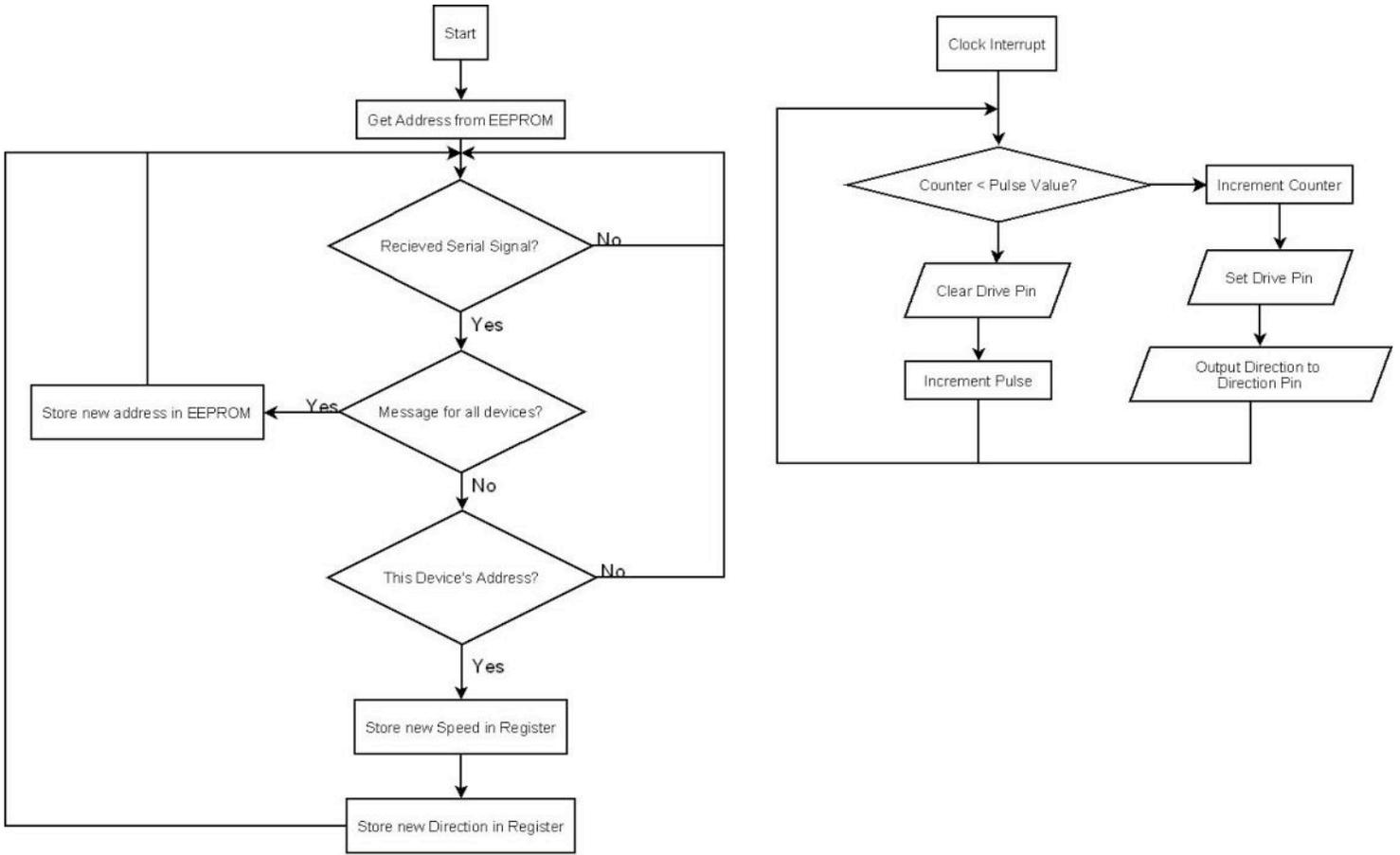
Figure C2. PIC microcontroller flowchart.
