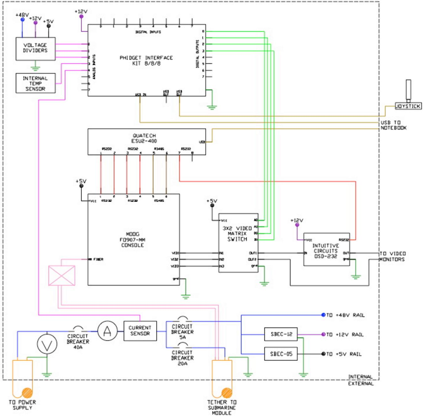
Figure B1. Schematic of topside control unit.
