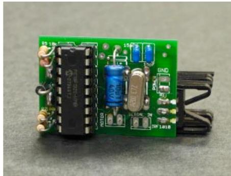
Figure 14. Embedded motor controller.
