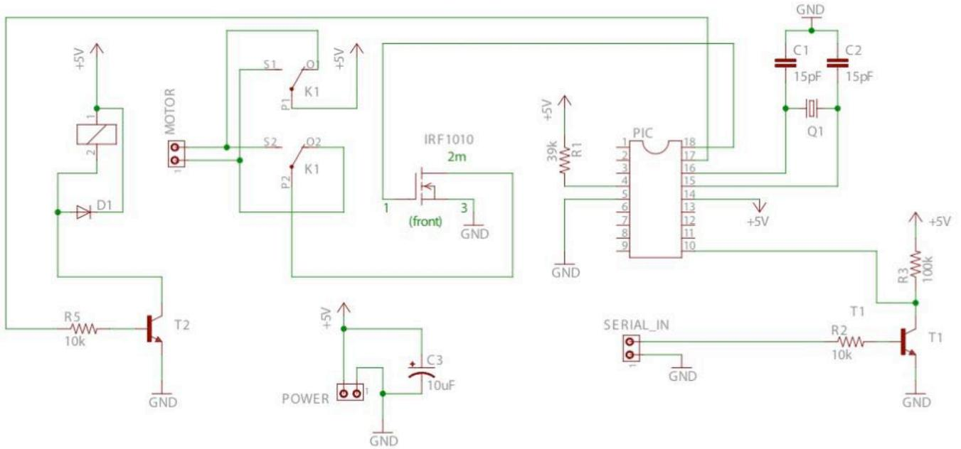
Figure B3. Schematic of embedded motor controllers.
