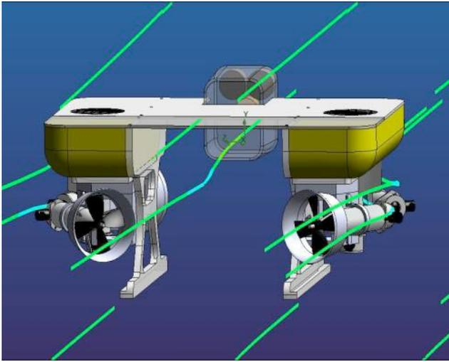
Figure A1. Flow trajectory of fluid particles as the ROV surges forward at 0.25 m/s.
