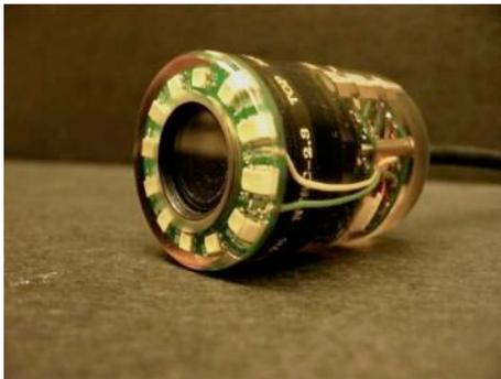
Figure 5. PCB camera.
