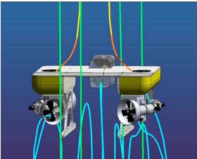
Figure A2. Flow trajectory of the fluid particles as the ROV heaves up at 0.25 m/s.
