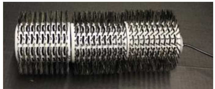
Figure 16. Brush biological sample collector.
