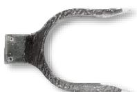
**Bident:** Resembling the Company's trident logo, the Bident is used to pick up and install the fountain heads. This tool is custom manufactured to fit the size of the object being handled. In the case of the 2017 contract, it is used to manipulate the fountain head.
