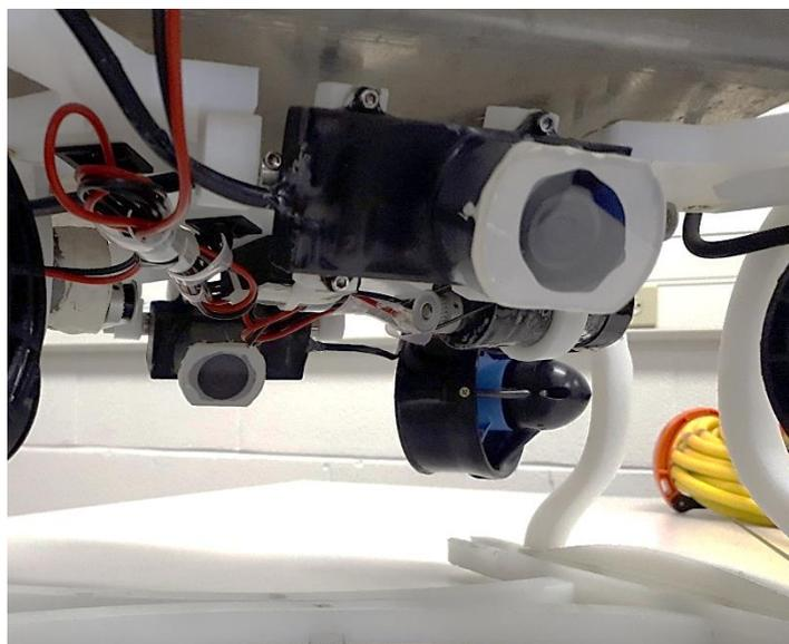
*Figure 9: Vimy's Camera System Attached to Chassis*
