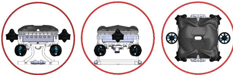
*Figure 3: CAD Rendering of Vimy with a 580 mm Diameter Circle in Each Axis*
