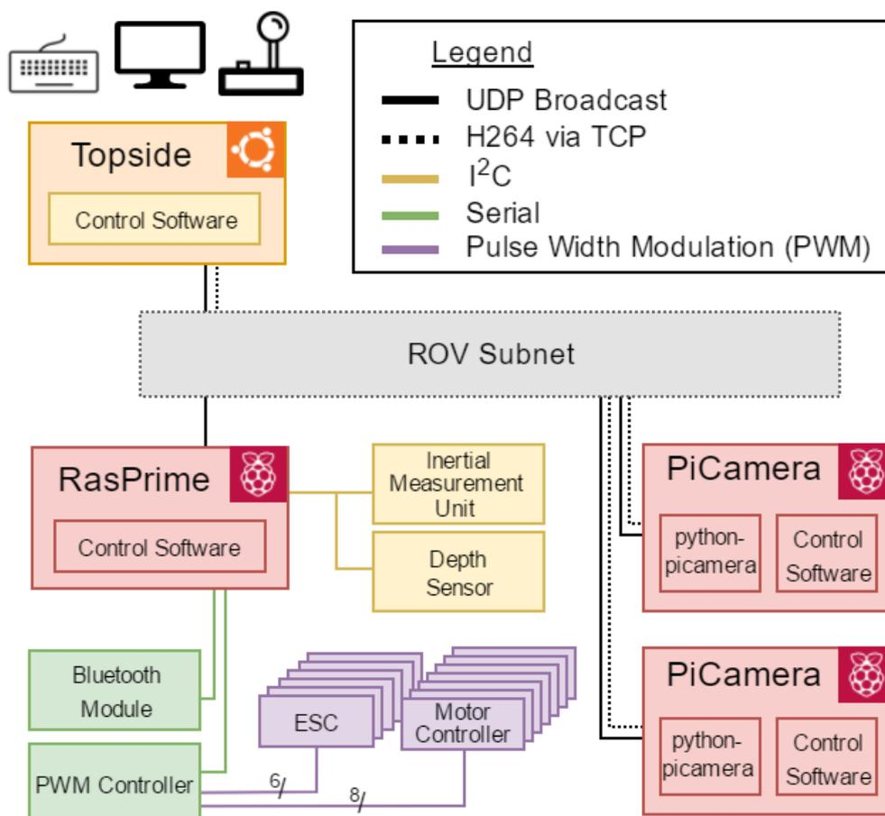
Figure 16: Software Communications Block Diagram
