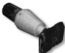
**M<sup>3</sup> (Magnetic Motor Mover):** The M<sup>3</sup> is one of two actuated tools on Vimy. M<sup>3</sup> is a bidirectional motor with a series of magnets placed on the rotation mechanism. This multipurpose tool is used to spin valves, move rebar and perform other miscellaneous tasks.
