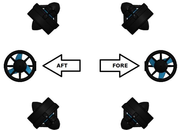
Figure 6: CAD Rendering of Thruster Layout
