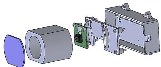
Figure 7: Exploded View of Vimy's Camera Module
