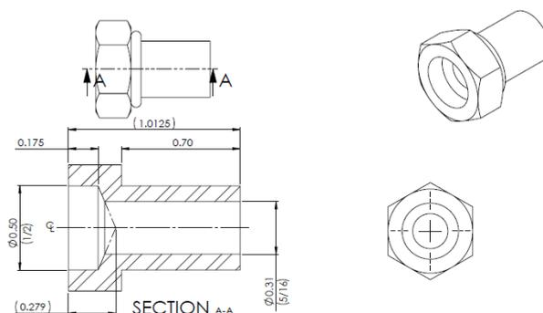
Figure 11: Custom Machined Penetrator
