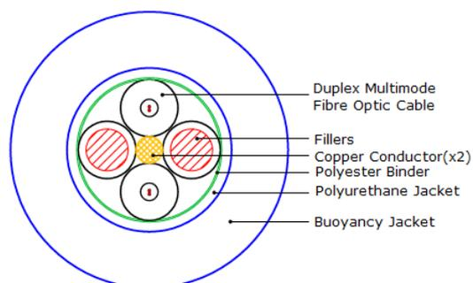
Figure 14: Tether Cross Section View
