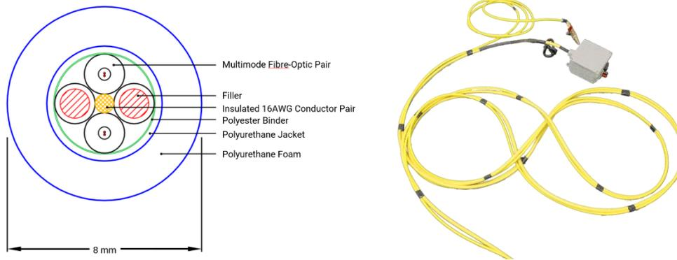
Figure 9: (Left) Cross Section of Tether. (Right) Tether and Pneumatic Tubing
